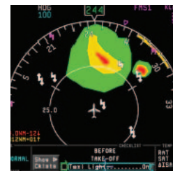
Lightning detection system
